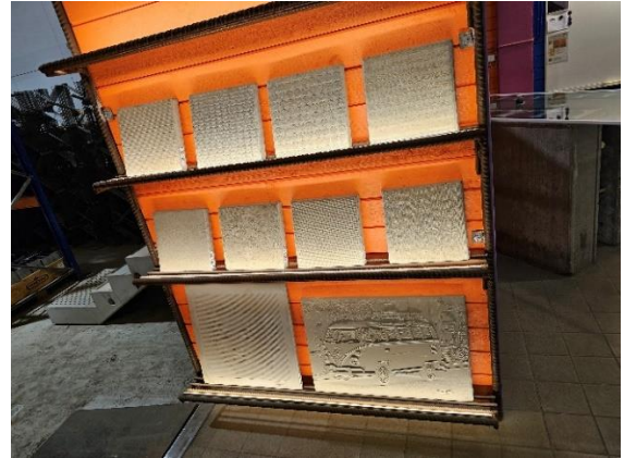
Figure 31: Pattern designs for prefabricated elements at Veidekke Prefab. Taken on 05.02.2024, at Klepp
