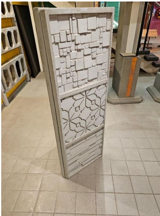
Figure 32: Pattern design for prefabricated elements at Veidekke Prefab. Taken on 05.02.2024, at Klepp
