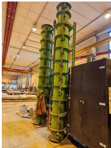
Figure 10: A long circular column mould. Taken on 05.02.2024, at Klepp
