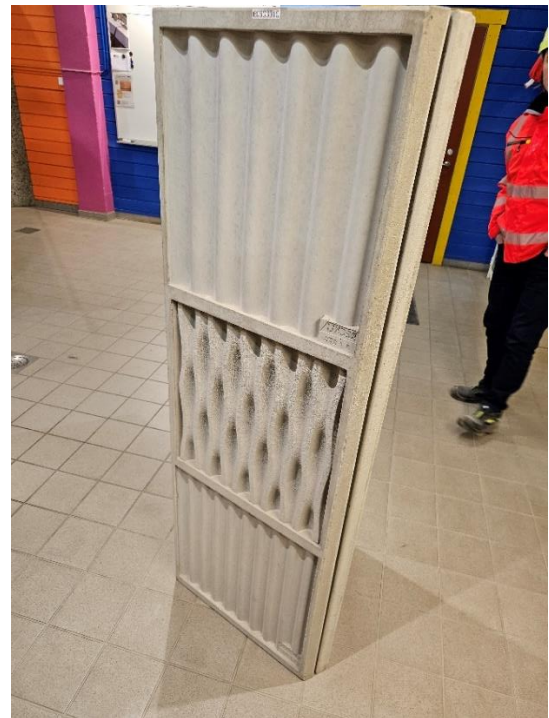
Figure 33: Pattern design for prefabricated elements at Veidekke Prefab. Taken on 05.02.2024, at Klepp
