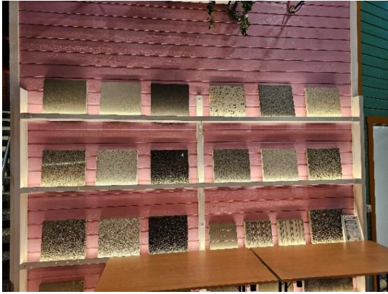
Figure 30: Outside finished for prefabricated elements at Veidekke Prefab. Taken on 05.02.2024, at Klepp
