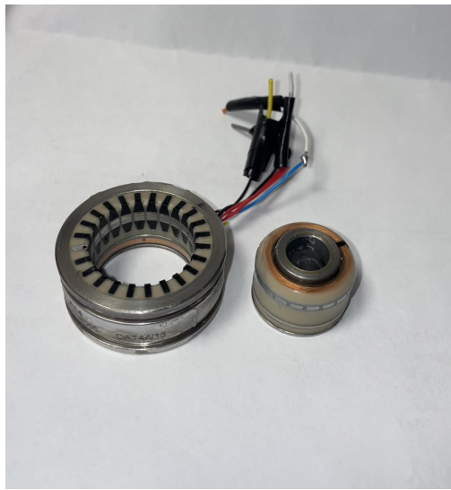
(a) Resolver: LTE Servotechnik RE-15.
