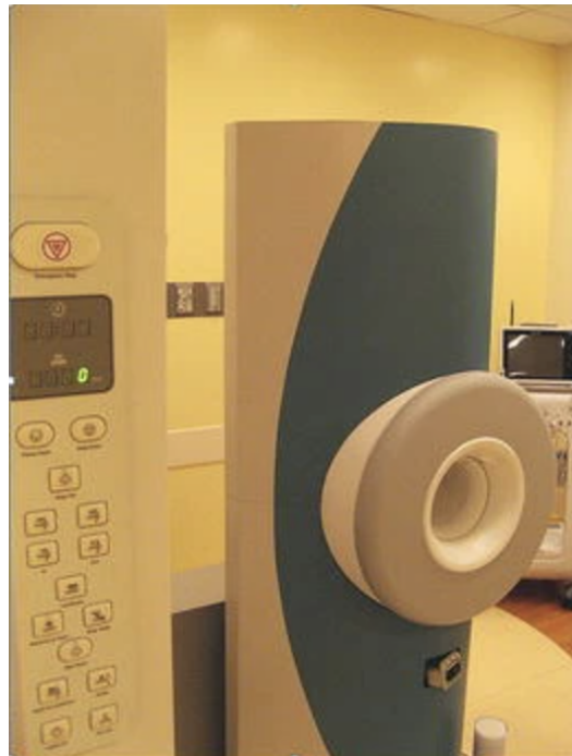
Figure 2.2: Image of the 1.5T OPTIMA MRI system post-adjustment for neonatal imaging. Adjustments to the OPTIMA system during the sheep studies involved raising the magnet's height and aligning it horizontally. Illustration is taken from [34] with permission
