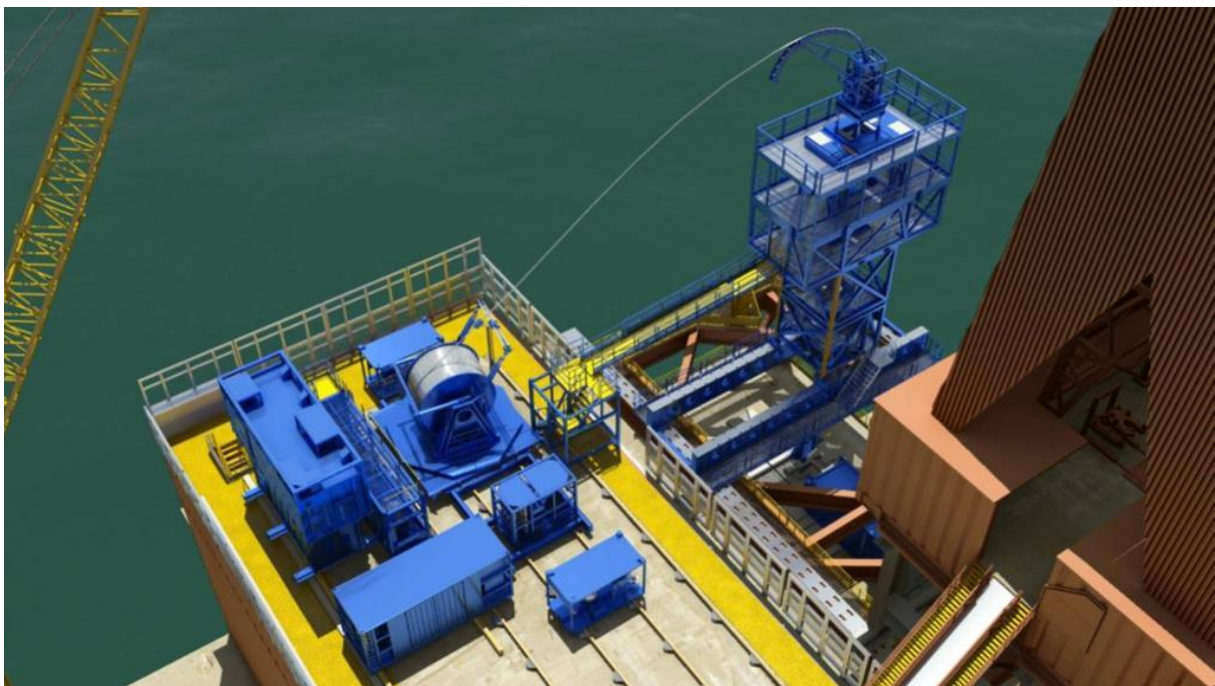
Figure 3 - Coiled Tubing Setup on the Well [7]
