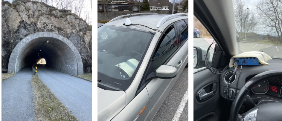
(a) Tunnel entrance, at the bottom of the hill in Skaarlia. (b) GNSS antenna placed on the roof of the car. (c) OBU mounted in the car. Powered by the car with an OBD2 connector.
