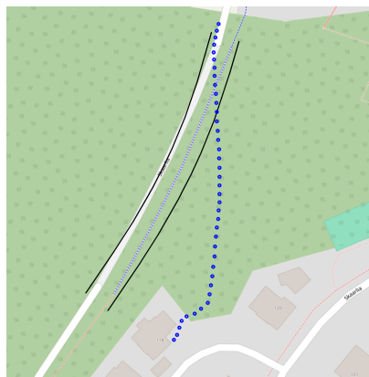
(a) GNSS from one dynamic measurement plotted on a map. The blue dots are the Lat/Lon coordinates, and the black lines are the estimated tunnel walls. Created using the OpenStreetMap database [50].
