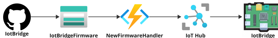
Figure 4.5: Github builds and releases a new version to the firmware blob container where it gets picked up by the NewFirmwareHandler and notifies the IoT-bridge devices
