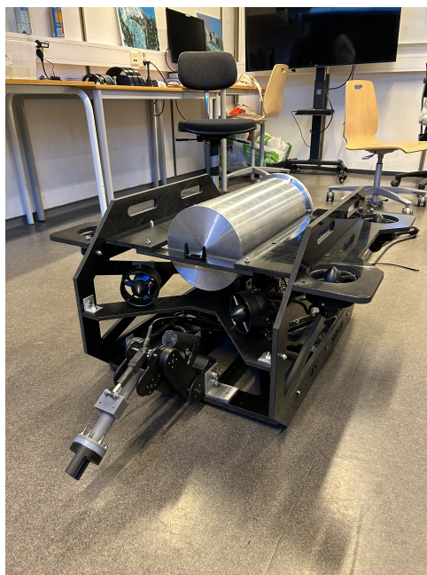
Figure 7.10: ROV-assembly for underwater test
