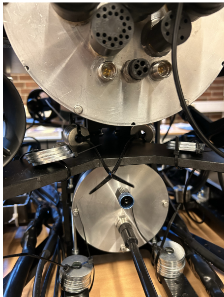
(a) Ballast installation on the rear end
