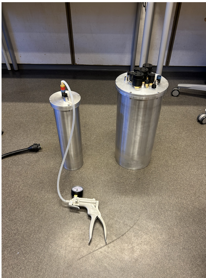
Figure 7.6: Vacuum test of the enclosures
