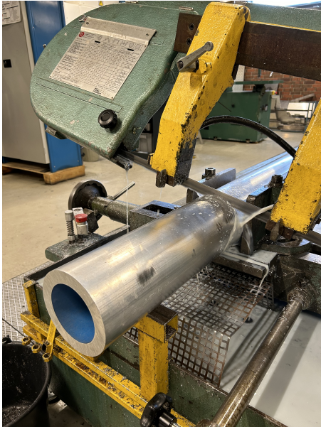
(a) Trimming the battery enclosure
