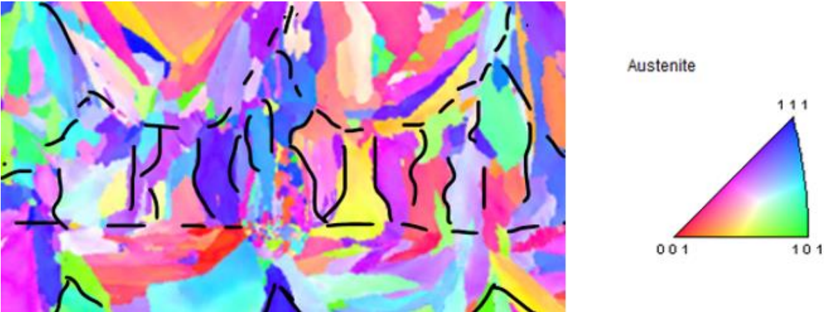
Figure 22: From sample B10, visible columnar grains overlapping the fusion boundary due to epitaxial solidification.
