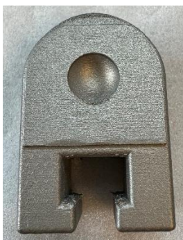
Figure 4-12 a) Printed wedge, b) Printed wedge with raised face
