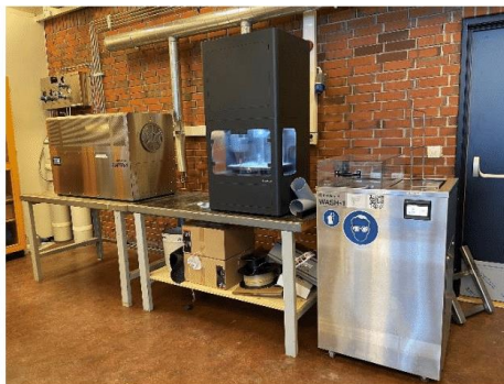
Figure 27 Markforged Metal X, WASH-1, and SINTER-1
