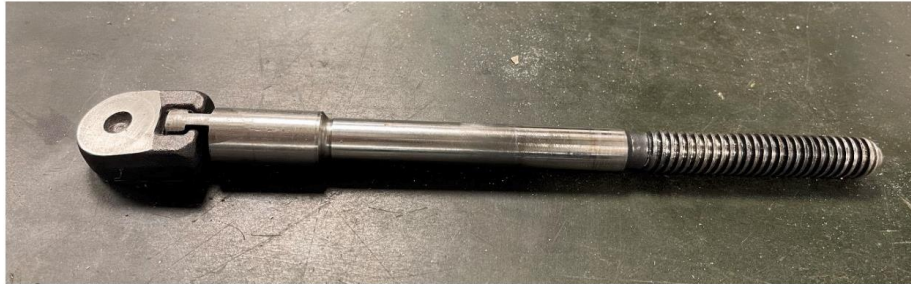
Figure 16 Valve wedge attached to stem rod
