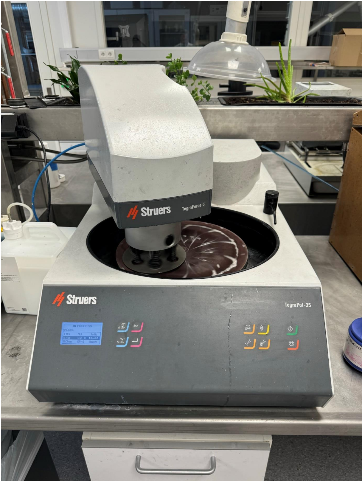
APPENDIX F - 10 Struers tegraforce-5 polishing machine
