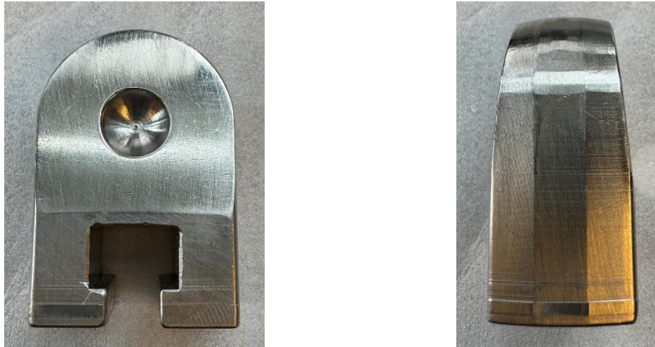
Figure 4-8 Subtractive manufactured wedge part
