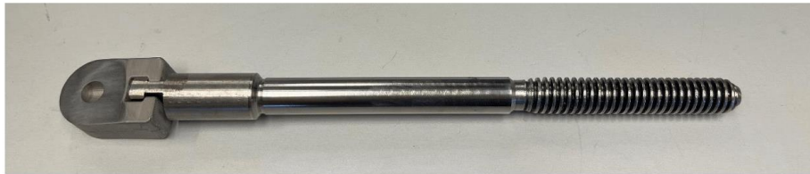
Figure 26 Printed part fitted on stem rod
