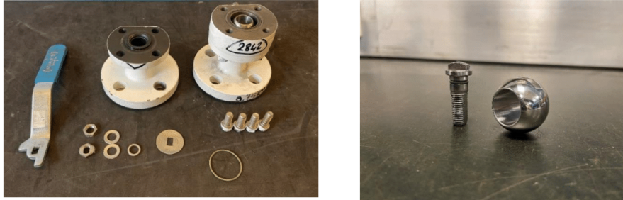
Figure 15 Ball valve dismantled.
