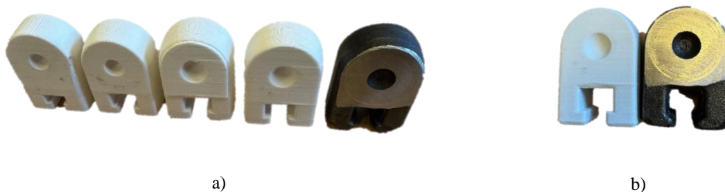
Figure 4-7 a) Prototypes and OE, b) Final design and OE
