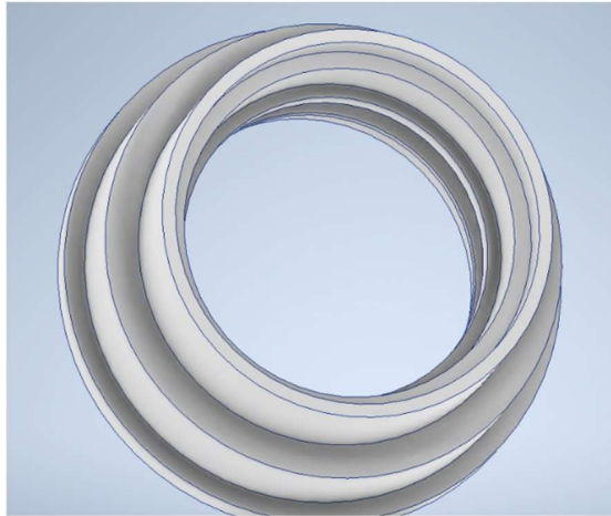
Figure 3.1.4 illustrates the hub requirements from the concept phase. This is the required material dimensions. The reason for the bigger diameter inside is to accommodate for the gearing which will be inside the upright.
