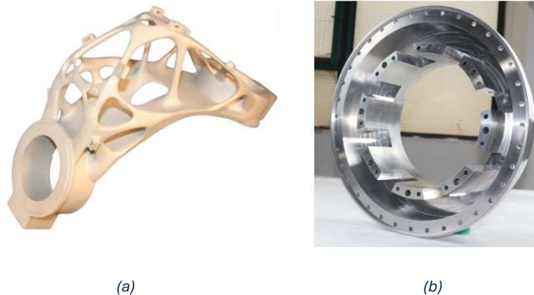
Figure 2.4.1 illustrates the difference in possibilities between additive manufacturing in part a on the left and traditional machining on the right in Figure (b). Figure (a) is a complex organic shape which would not be able to produce with traditional manufacturing because the tools would not get access to all the mass that must be removed. In contrast, Figure (b) has straight edges and is therefore possible to manufacture by subtracting the unnecessary mass (In3dtec, 2024) (In3dtec, 2024).
