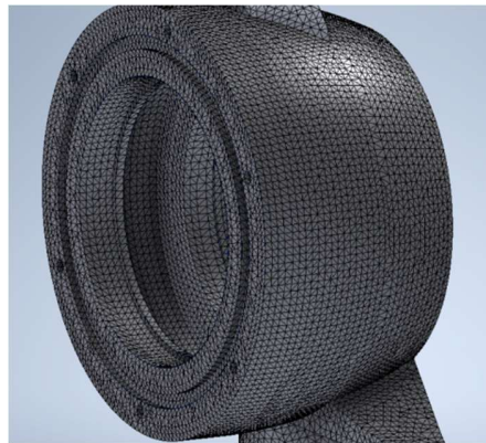
Figure 2.3.4 illustrates the upright part with mesh. The black lines over the part are the mesh. This is the Upright in the concept development of this project and the mesh is used in the simulation at that stage.
