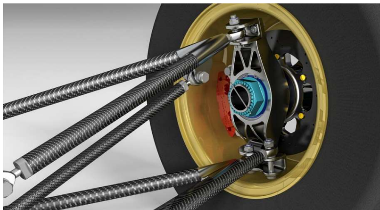
Figure 2.1.1 Shows an example wheel assembly from a formula student car (grabcad.com, 2024).
