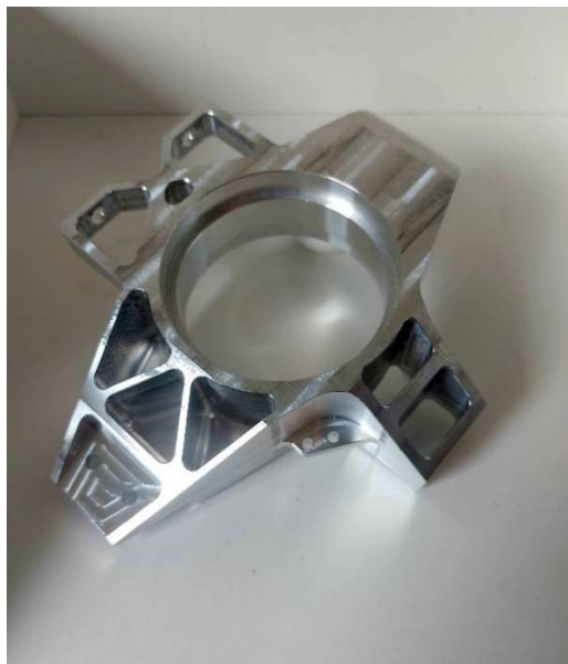
Figure 2.1.3 Picture of previously used up-right by ION-racing. This design was basic but effective. As well as being flexible. However, due to changing criteria from ION racing it is no longer suitable.
