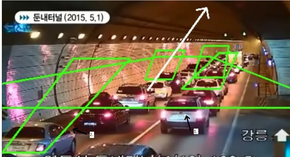
Figure 4.4: The figure is showing a failed queue detection with the queues labeled 1 and 2 being the main focus.
