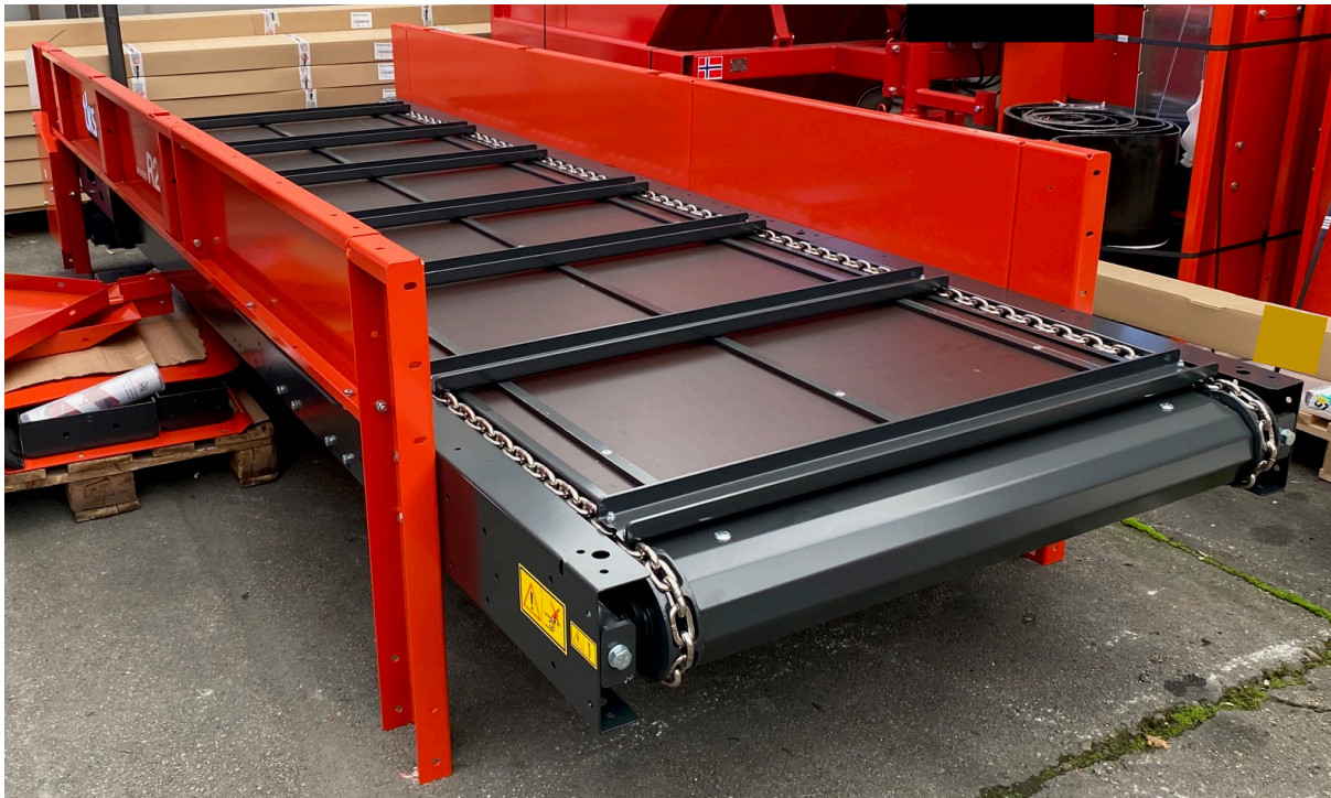
Figure 1.3 R2 Magazine with a long version of the frame. Otherwise similar to the frame on K2 CombiCutter. Private photo.
