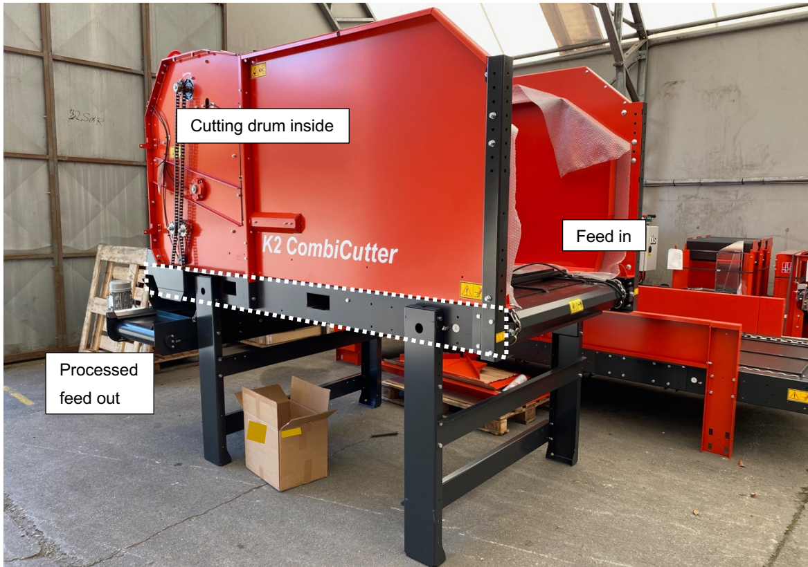
Figure 1.1 K2 CombiCutter. Side plate of frame highlighted with stapled white lines. Private photo.
