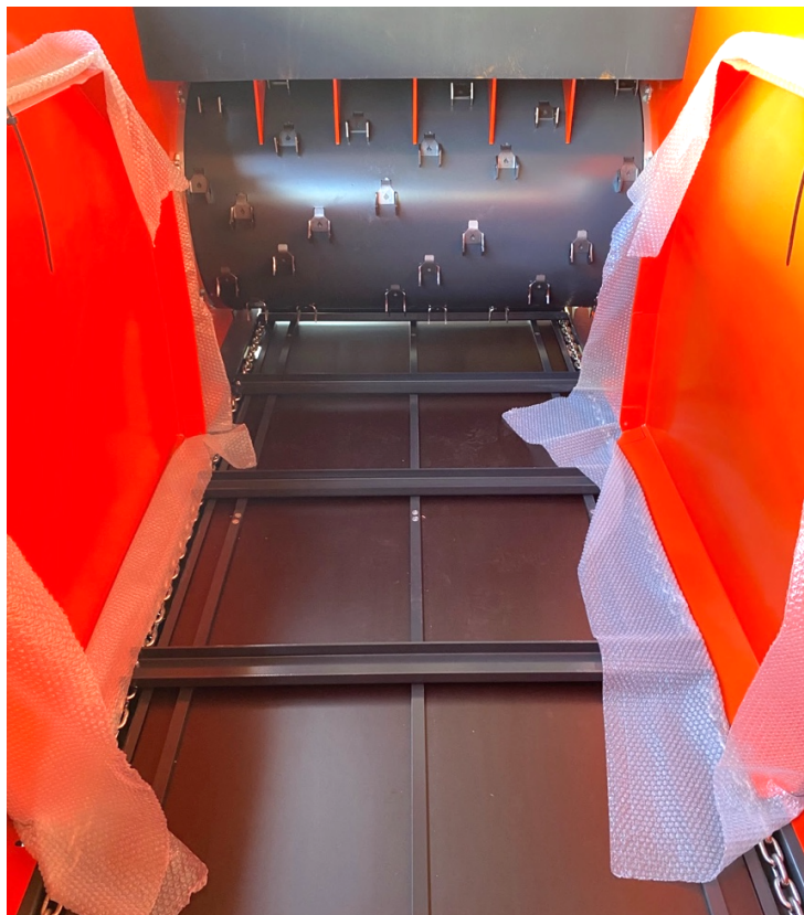
Figure 1.2 Inside K2 CombiCutter. Grey cutting drum with knives. The floor is the top of the frame. Chain-driven transport function which moves the feed towards the drum. Private photo.
