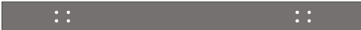
Figure 3.4.1 Diagram showing bolt holes in the outer side of the frame where fixed supports are applied to simulate floor stands
