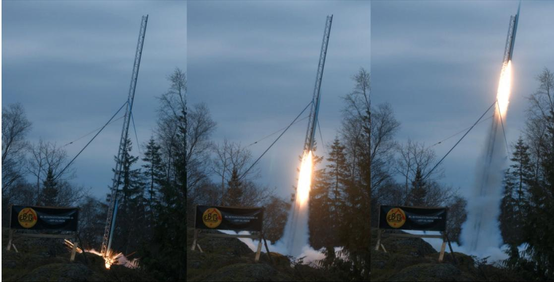
Figure 1.4: Borealis accelerates along the 15 meter long launch rail at Helleland.
