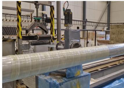
Figure 8.5: Wet winding
