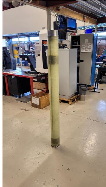
Figure 8.8: Assembled middle fuselage before painting
