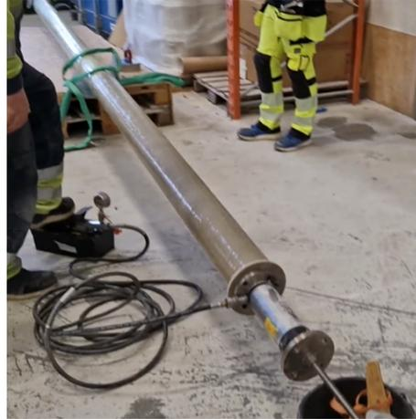
Figure 8.7: Hydraulic jack extraction
