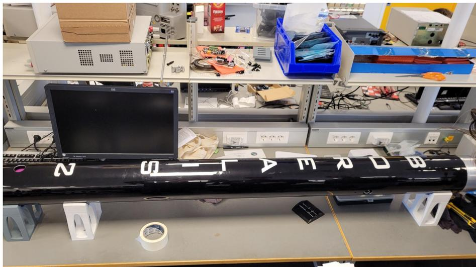
Figure 8.9: Assembled middle fuselage after painting
