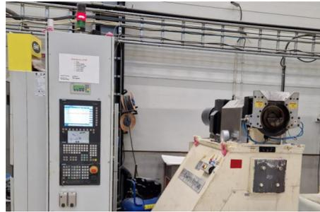
Figure 8.3: Control panel for winding machine
