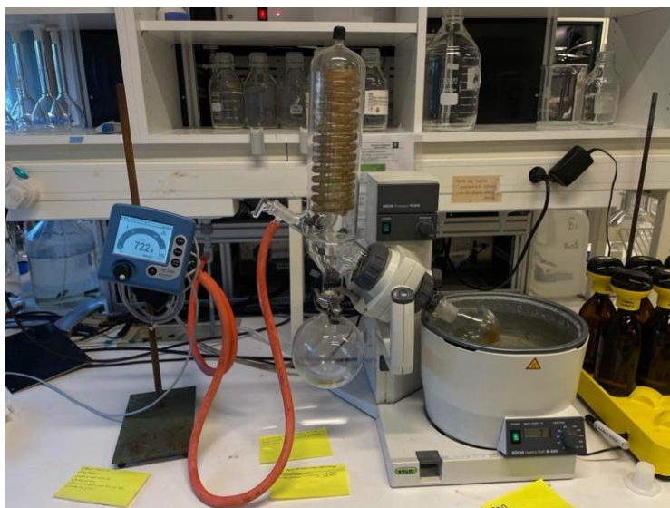
Figure 4.6 Setup for Rotavapor R-200.
