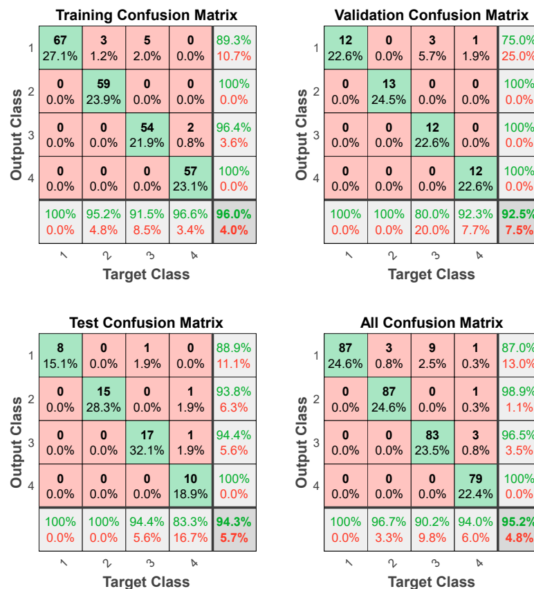
Figure 12. Confusion matrix for the fault detection and isolation during the NG-fueled scenario.
