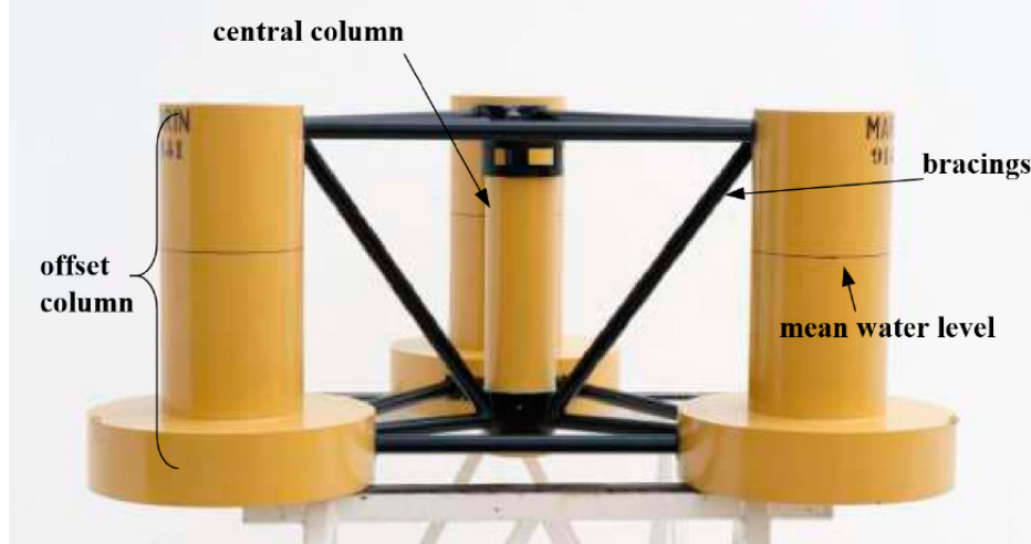
Figure5. 1/50 scale model of the DeepCwind semi-submersible platform.
