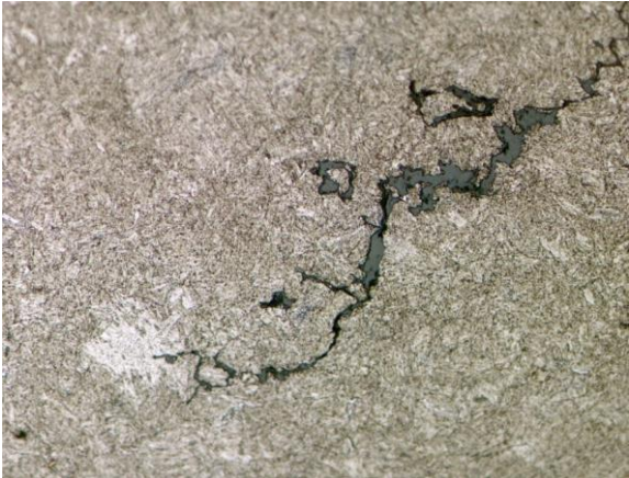
Figure 33 FAH-2 50X possible ductile crack growth.
