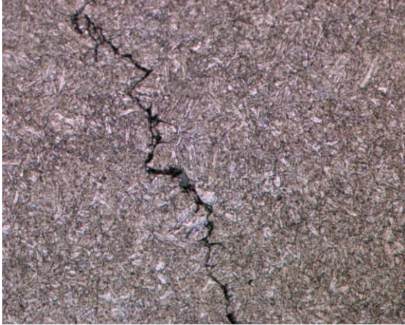
Figure 35 FCH-1 50X possible ductile crack, zig zag pattern.
