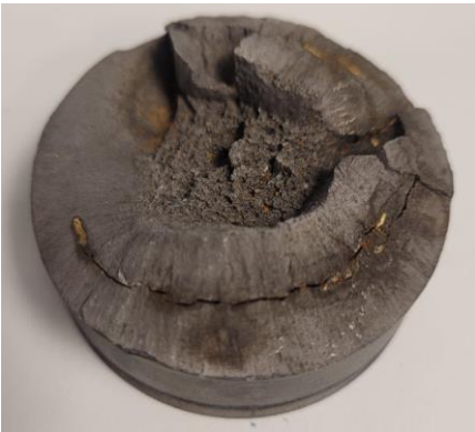
Figure 30 Fracture surface bolt A.
