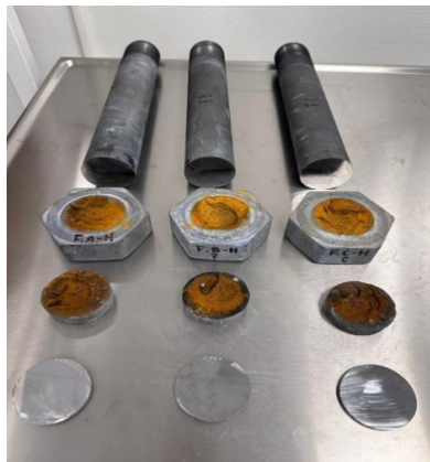
Figure 20 Overview of shanks, bolt heads, fracture surfaces and shank specimens.
