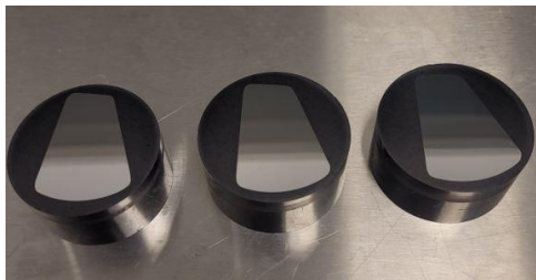
Figure 24 Finished mounted specimens from bolt shanks.
