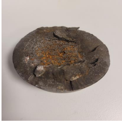
Figure 31 Fracture surface bolt C
