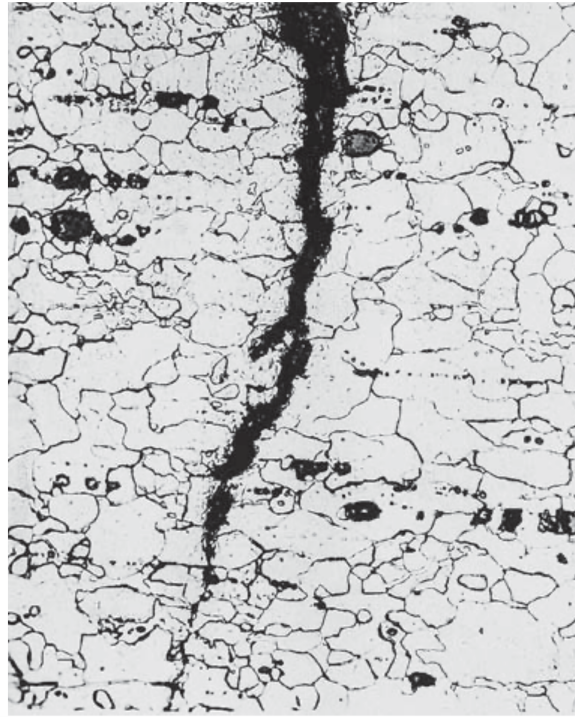
Figure 2.7: Corrosion-fatigue crack in mild steel sheet (250x) [14]
