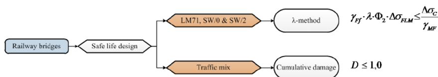
Figure 3.4: Fatigue Load Model for railway bridges [30]
