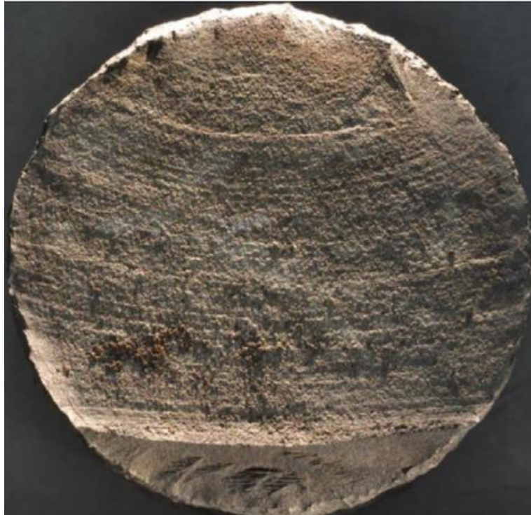
Figure 3.13 Fatigue crack growth and beach marks formation on a mooring chain cross section reproduced from [57].
