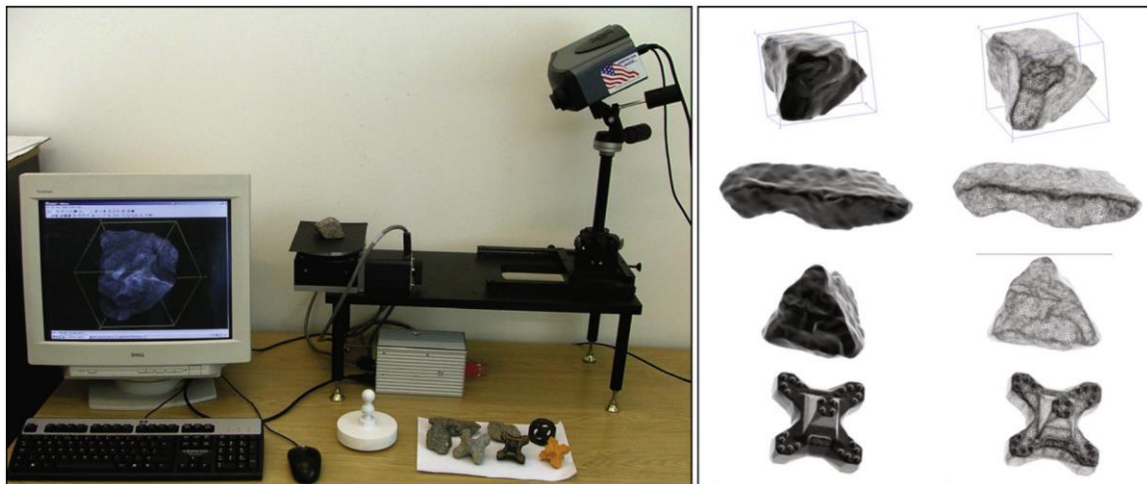
Figure 3.14: 3D image capture system for high resolution 3D images of rock (Latham et al., 2008)
