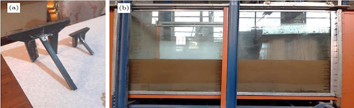
Figure 3.9: Experimental setup used by M. Naeij to study anchor interaction with trenchless pipeline covered with backfilled soil and rock berm (Naeij et al., 2023)
