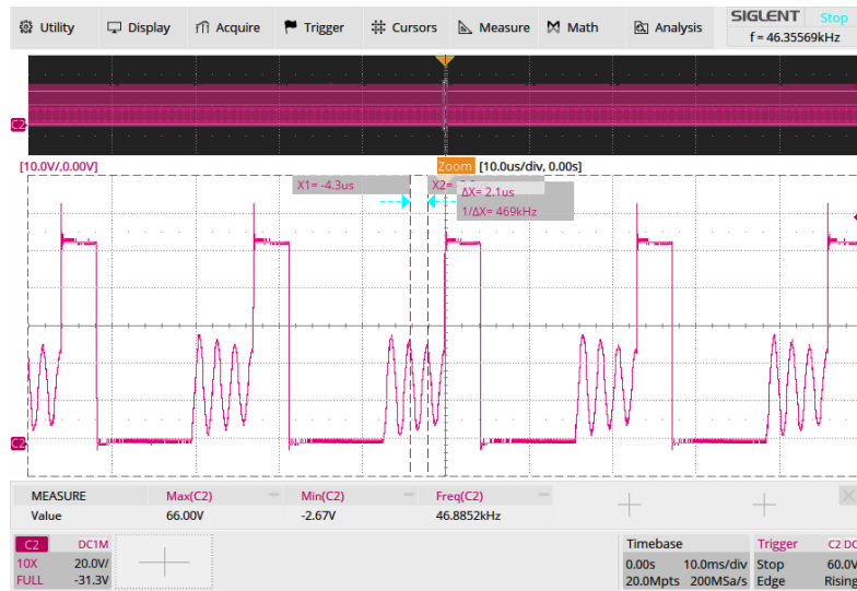
Figure 4.2.4: Synchronous rectifier voltage at normal operation.
