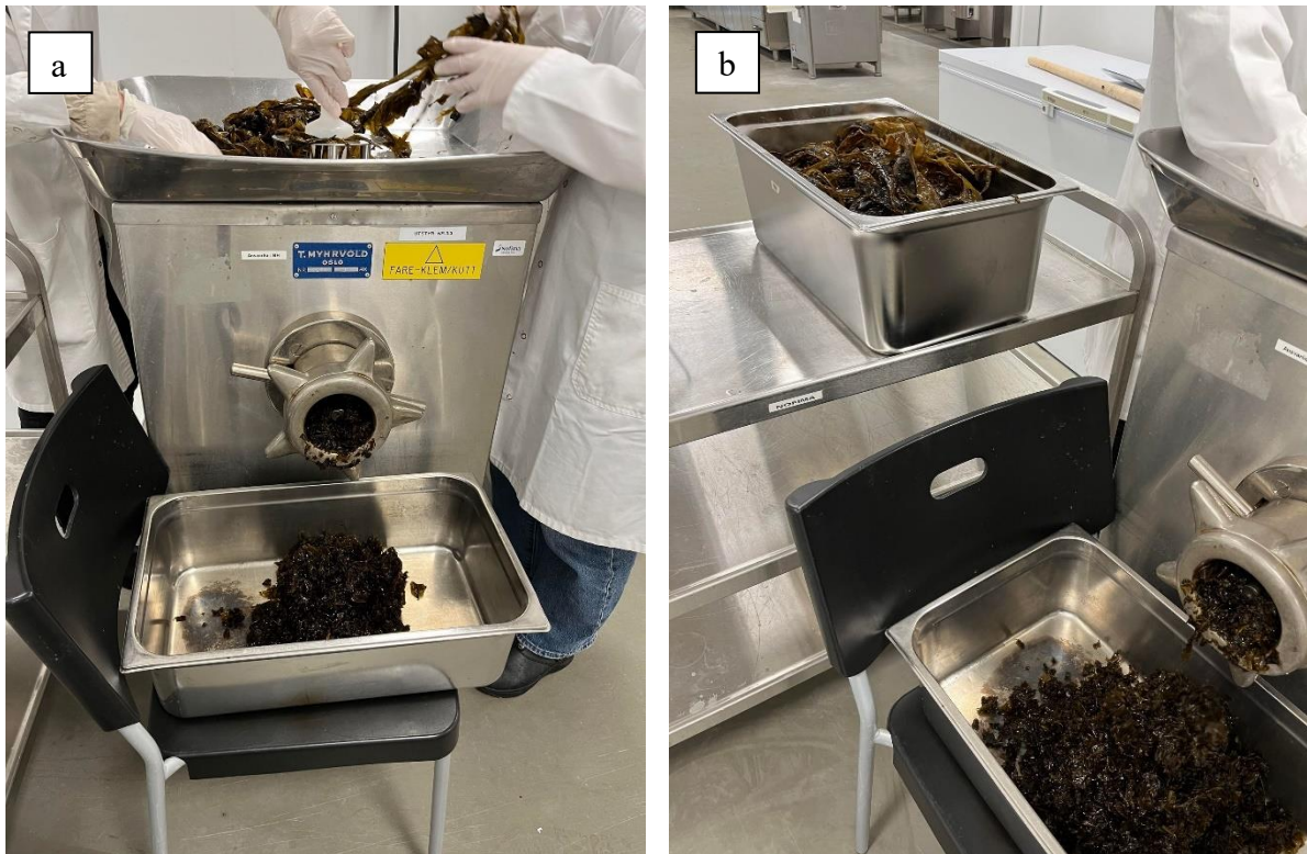
Figure 2.10: Picture of (a) grinding process and (b) showing the difference between whole and grounded winged kelp.
