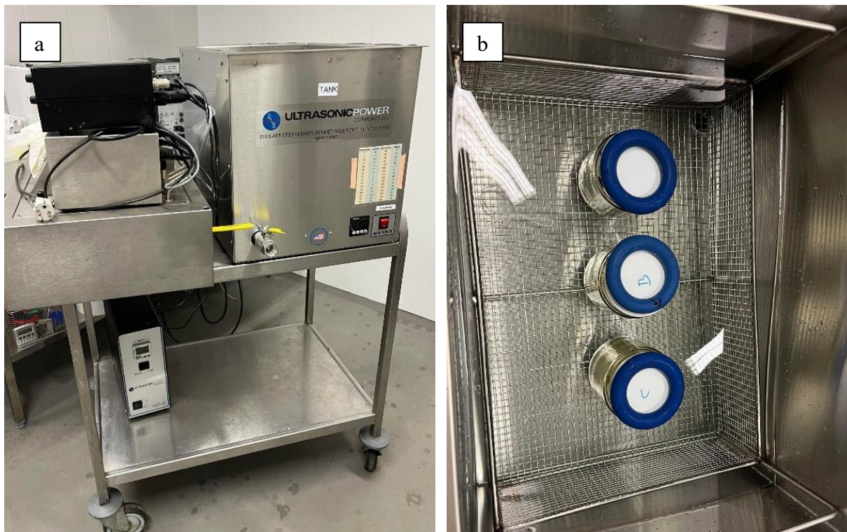
Figure 2.11: (a) Ultrasonic Power Corporation Ultrasonic cleaner with one generator on the bottom shelf and (b) samples of rockweed and tap water in glass jars, placed in a mesh basket, and held under water with weights.
