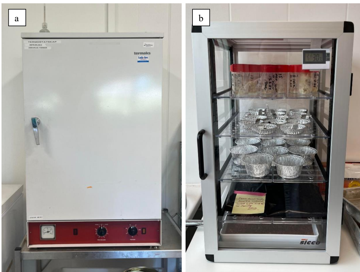
Figure 2.17: (a) Termaks T1056 (Nordic Labtech, Sweden) and (b) Star-Vitrum desiccator (Sicco, Denmark).
