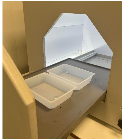
Figure 2.16: Transparent white plates in the DigiEye instrument.
