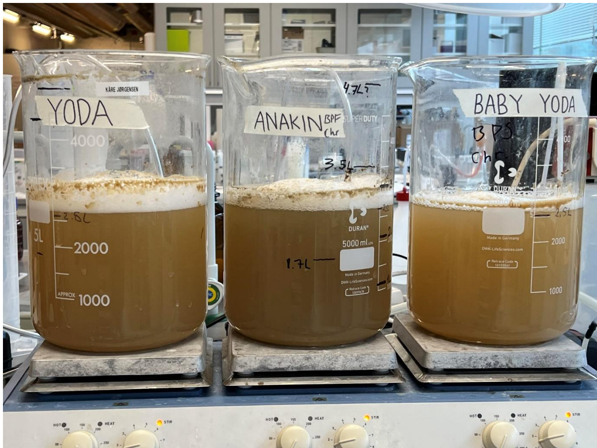
Figure 12 – Photograph of the chronic BPA (Left), BPF (Middle) and BPS (Right) reactors
